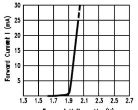
Forward Voltage V<sub>F</sub> (V) Fig.2 Forward Current vs. Forward Voltage
